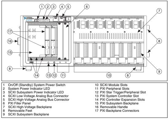
Figure 1-1. Front View of the PXI-1052 Chassis
